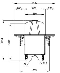
D = Drain El = Electrical inlet (power)
